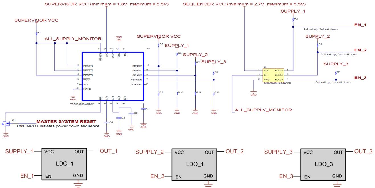
Figure 1. Sequencing Supervisor Schematic
