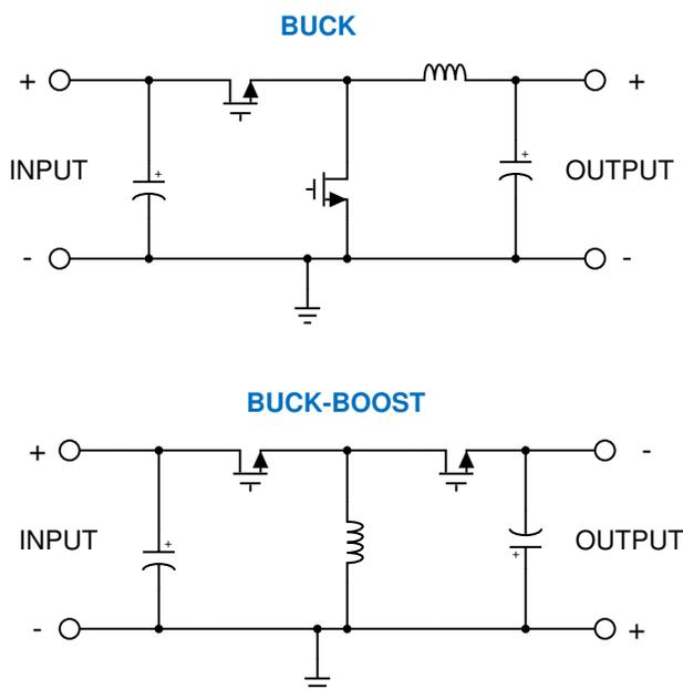
**Figure 2-1. Comparison of Buck and Inverting Buck-Boost Topology**
