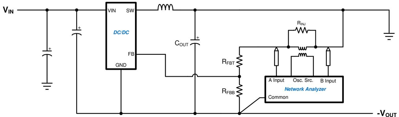
Figure 4-2. Set-up for Measuring Bode Plots for an IBB
