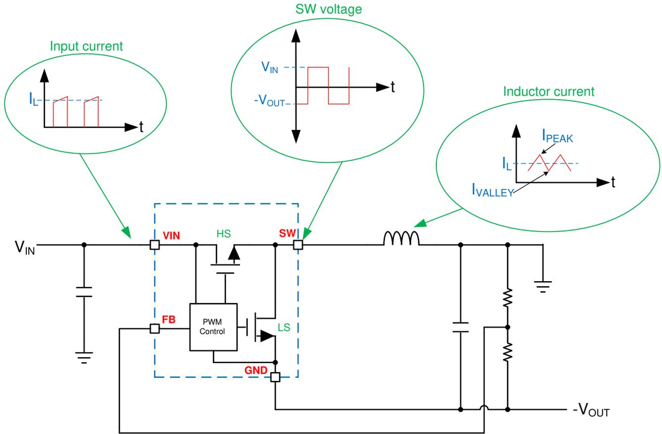
Figure 3-1. Inverting Buck-Boost Waveforms
