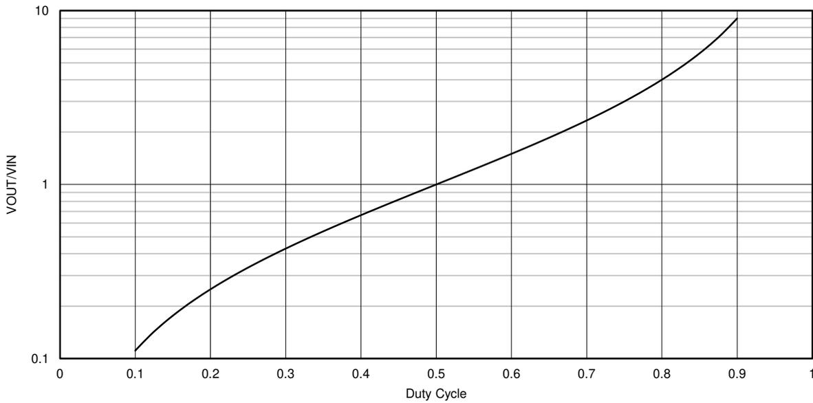
Figure 3-2. Conversion Ratio vs Duty Cycle
