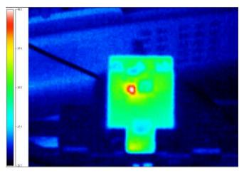
Figure 1. LM27402 Thermal Performance
