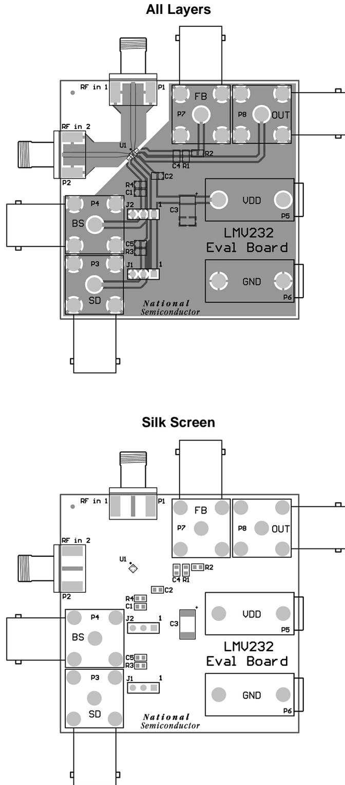
Figure 2. Layout of the Evaluation Board
