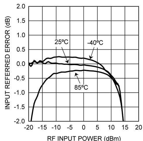
Figure 5. Input Referred Error vs. RF Input Power at 900 MHz
