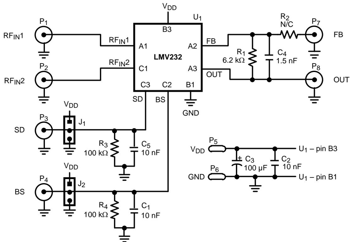
**Figure 1. Schematic of the Evaluation Board**
