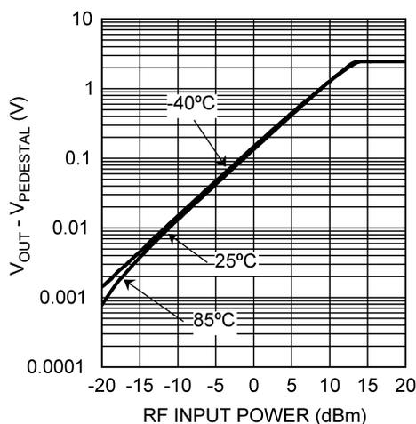
Figure 4.  $V_{OUT} - V_{PEDESTAL}$  vs. RF Input Power at 900 MHz
