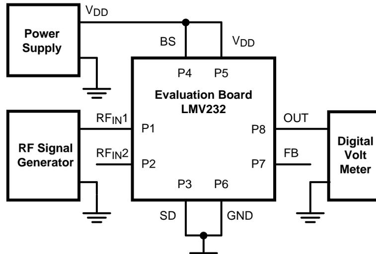
Figure 3. Measurement Setup
