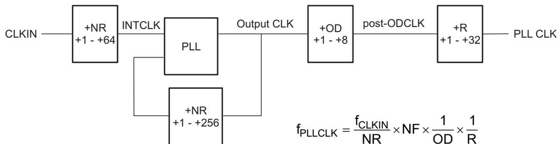
Figure 1. PLL Block Diagram
