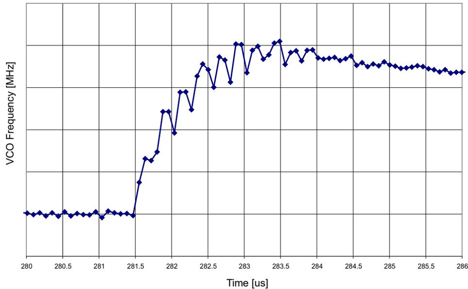
**Figure 2. PLL CLK Frequency Step With a Multiplier Change**
