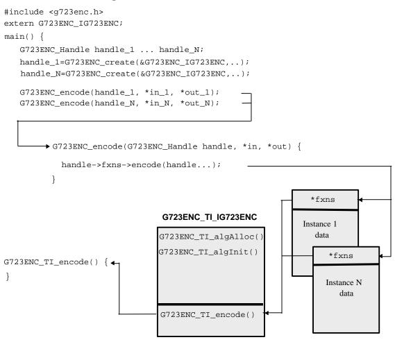
Figure 4. Example of a Multichannel System With TI G.723.1 Encoder Modules
