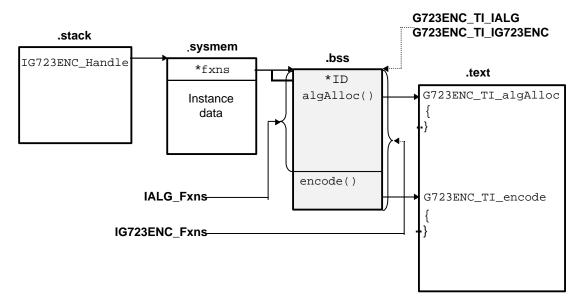
Figure 2. TMS320 DSP Algorithm Standard Structure
