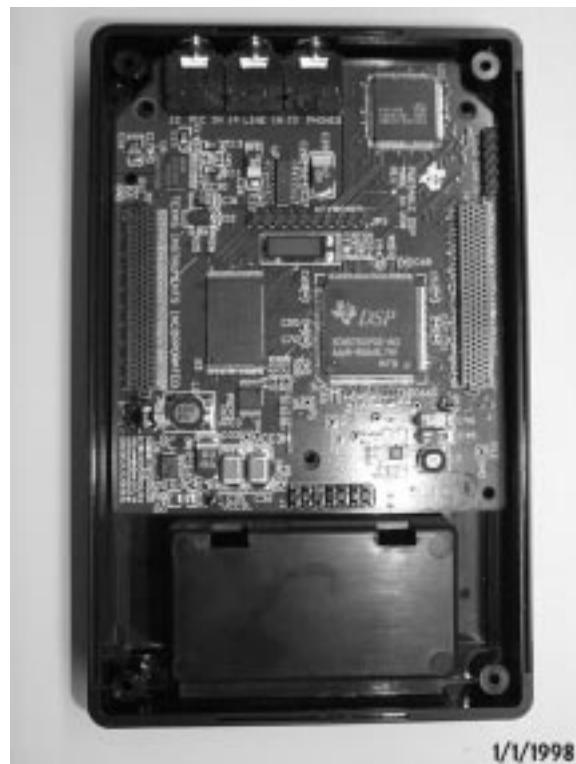
Figure 12. Battery Powered Hearing Aid Prototyping System (5.75" x 3.69" x 1.29", 5 ounces, 232mW)
