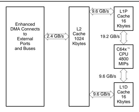
Figure 1. C64x Two-Level Cache Architecture
