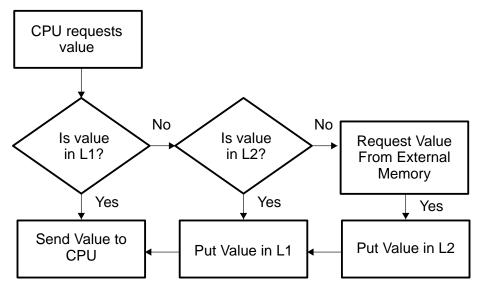
Figure 2. C64x Two-Level Cache Fetch Flow
