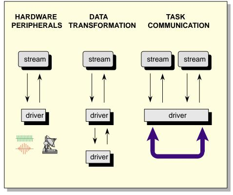
Figure 4. DSP/BIOS Streaming I/O Data Streams
