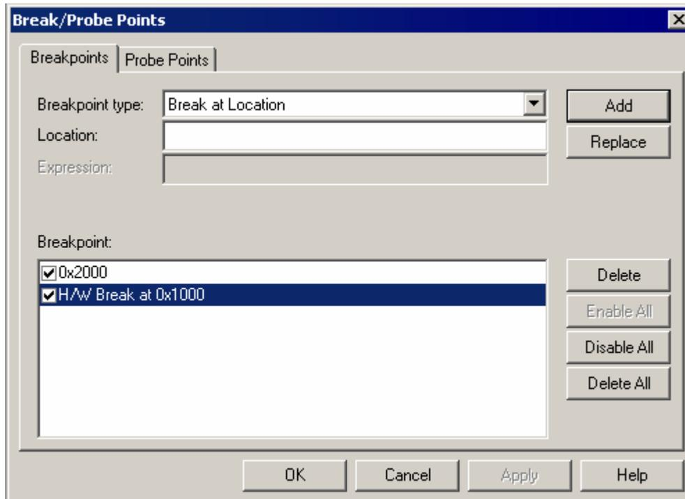
**Figure C-1. Hardware Breakpoints in Code Composer Studio v2.20**
