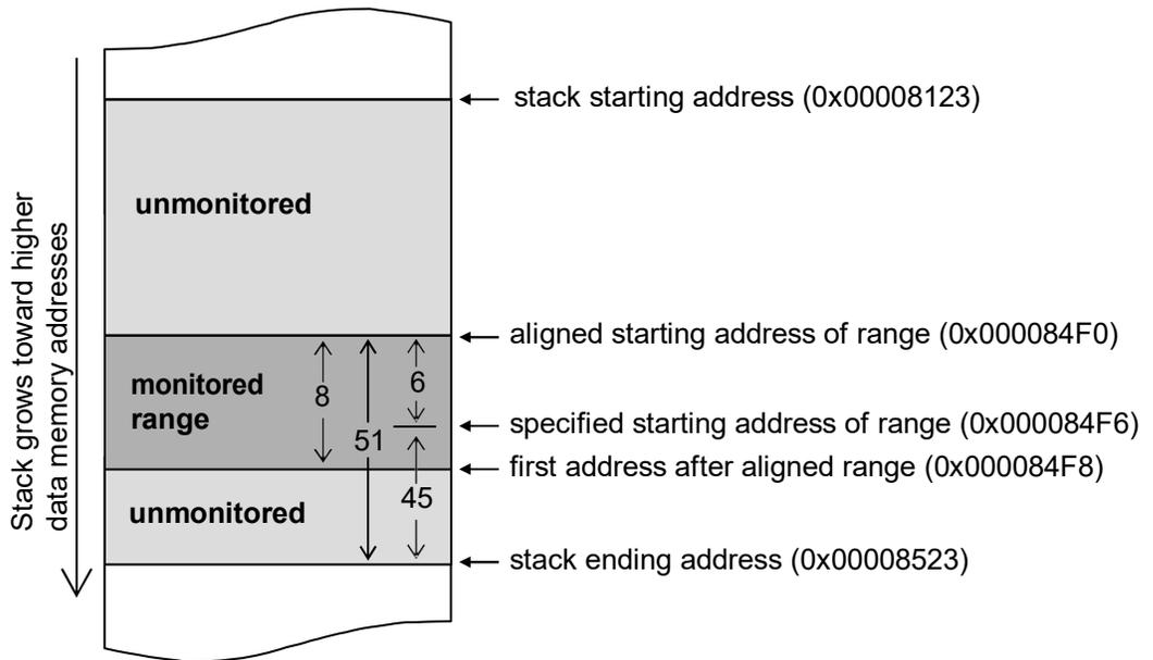
**Figure 2. Watchpoint Range in Relation to the Stack in Memory**
