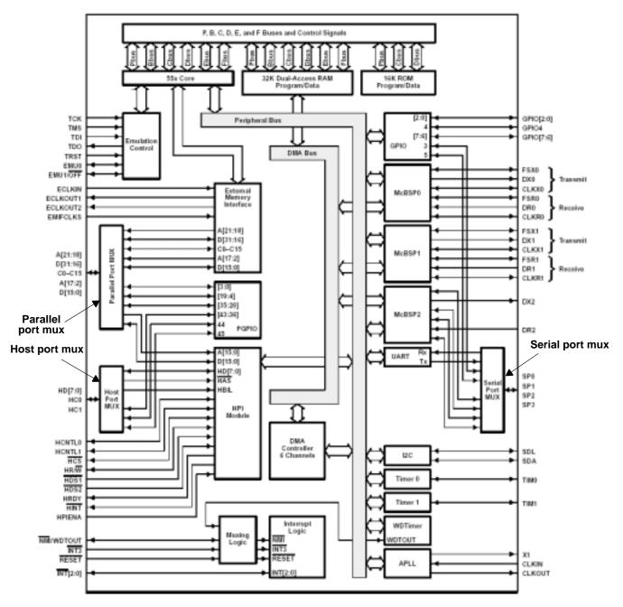
Figure 2. VC5502 Functional Diagram
