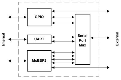
Figure 3. Serial Port Functional Diagram
