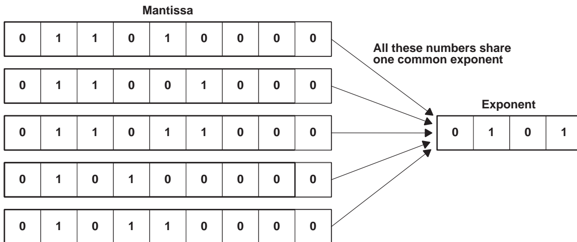
Figure 3. Diagram of Block Floating-Point Representation
