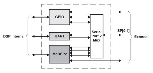
Figure 7. Serial Port 2 Mux Interface
