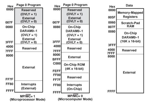
NOTE: Address ranges for on-chip DARAM in data memory are: DARAM0: 0080h-1FFFh; DARAM1: 2000h-3FFFh
