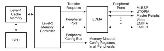
Figure 2. L2 Controller Functionality
