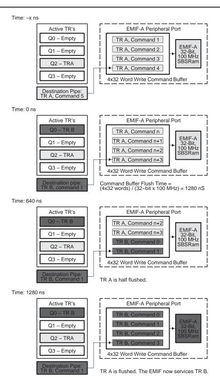
Figure 7. Example Port Blocking Scenario
