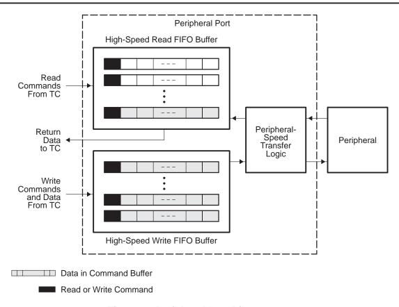
Figure 3. Peripheral Port Diagram
