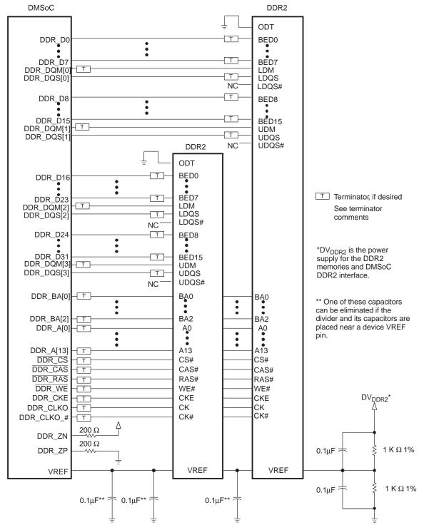
Figure 1. DM4xx DDR2 High Level Schematic
