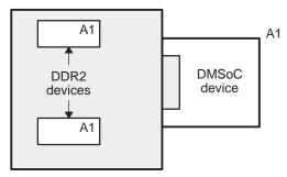
Example DDR2 keep-out region. Region should encompass all DDR2 circuitry and will vary depending on placement. Non-DDR2 signals shall not be routed on the DDR2 signal layers within the DDR2 keep-out region. Non-DDR2 signals may be routed in this region provided they are routed on layers separated from DDR2 signal layers by a ground layer. No breaks shall be allowed in the reference ground layers in this region. In addition the 1.8V power plane should cover the entire keep-out region.
