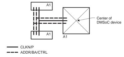
Figure 7. General Address, Bank Address, Control, and Clock Routing
