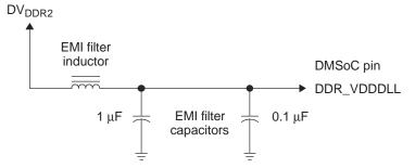
EMI filter capacitors should be placed no further than 350 mils from associated DMSoC ball.
