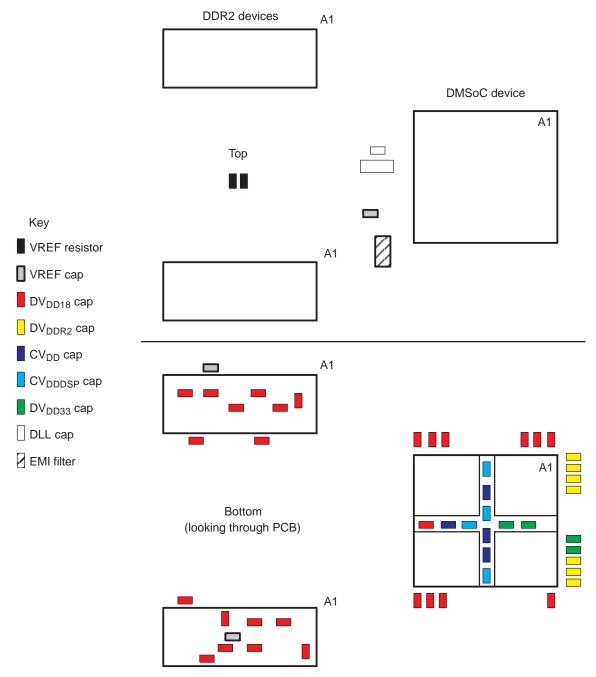
Figure 5. Discrete Part Placement
