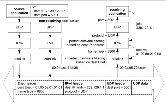
Similarly, to be able to send data to a multicast group, a host must create a UDP socket with the same port and group address as the listening socket. The same socket cannot be used to send and receive packets, since the IP standard forbids packets from having a multicast address as the source address.
