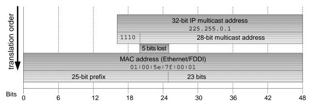
At the transport layer, both broadcast and multicast communications require UDP (User Datagram Protocol) or raw IP sockets to perform communications, since TCP is a connection-oriented protocol designed for use in point-to-point communications.
