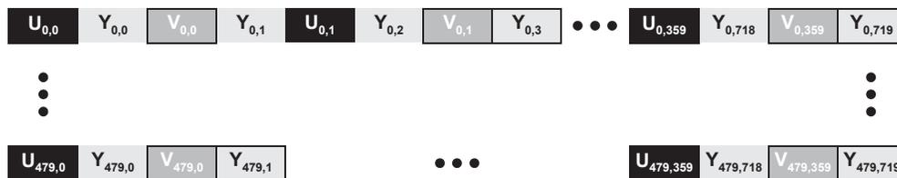
**Figure 3. NTSC D1 YUV422 Interleaved Format (UYVY)**
