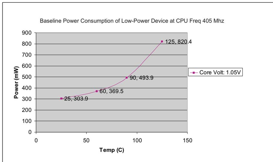
Figure 2. Baseline Power Consumption Across Voltage and Temperature: Low-Power
