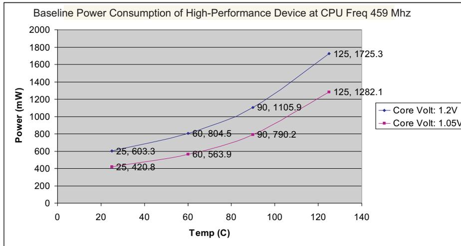
Figure 1. Baseline Power Consumption Across Voltage and Temperature: High-Performance
