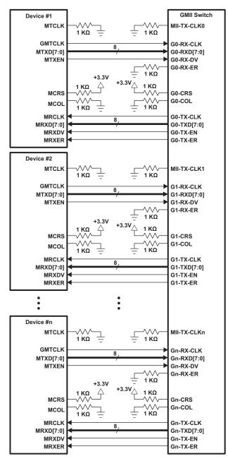
Figure 2. GMII Switch Connectivity Diagram
