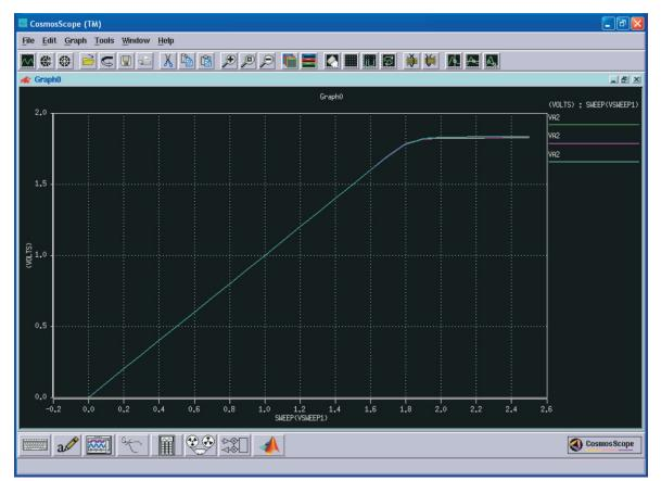
Setup for  $V_{OUT}$  vs.  $V_{IN}$  plot: B2 was swept from 0 to 2.5 V in 0.1-V steps and the waveform at A2 was observed. A 1MB resistor to GND was connected at A2.
