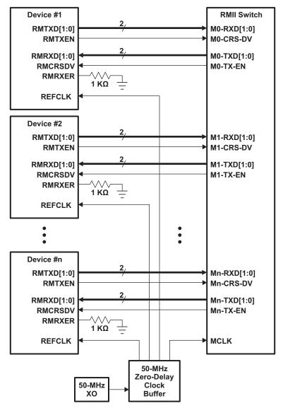
Figure 5. RMII Switch Connectivity Diagram
