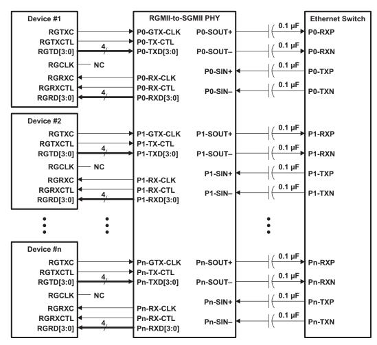
Figure 7. RGMII Switch Connectivity Diagram
