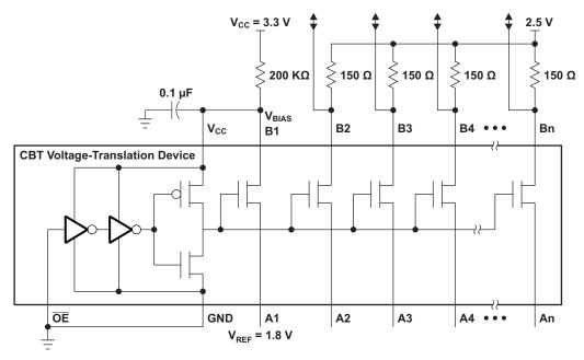
Figure 13. RGMII Voltage Level Translation Circuit
