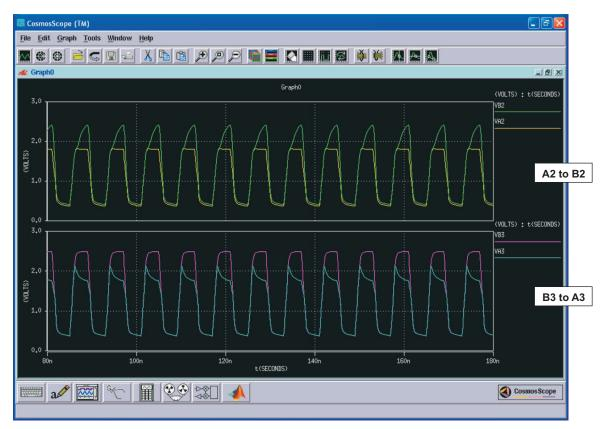
Figure 15. 125-MHz Signal From A2 to B2 and From B3 to A3
