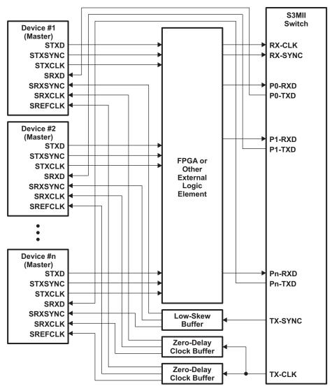
Figure 12. S3MII Multi-Switch Connectivity Diagram
