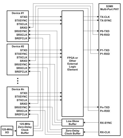
Figure 10. S3MII Multi-Port PHY Connectivity Diagram
