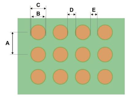
Figure 8. Recommendations for 0.4mm Pitch Packages - Top Layer
