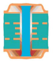
Figure 14. Plated, Filled and Capped BGA Pad
