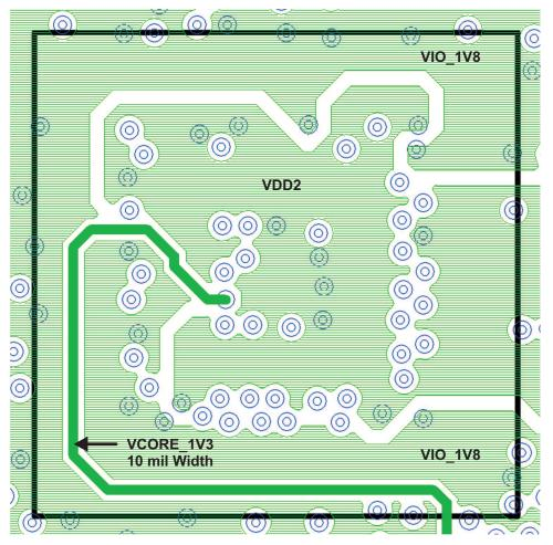
Figure 23. Close-Up of BeagleBoard Layer 5 - Power Plane
