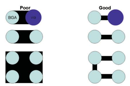
Figure 12. Common Sense Routing Circuit Board Guidelines
