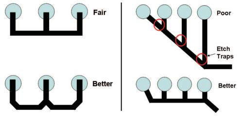
Figure 11. Common Sense Routing Circuit Board Guidelines
