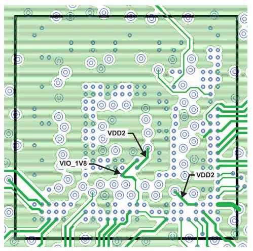
Figure 20. Close-Up of BeagleBoard Layer 2 - Ground Plane
