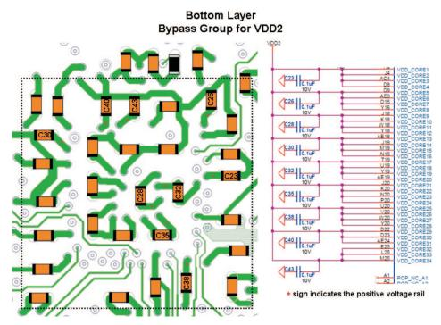
Figure 25. BeagleBoard Bypass Group for V<sub>DD2</sub>
