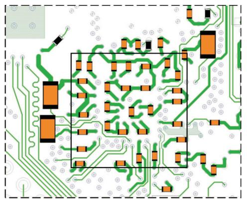
Figure 24. Close-Up of BeagleBoard Layer 6 - Bottom Side
