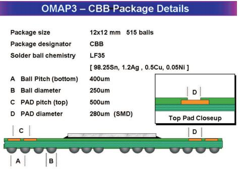
Figure 5. OMAP35x - CBB Package Specification Details
