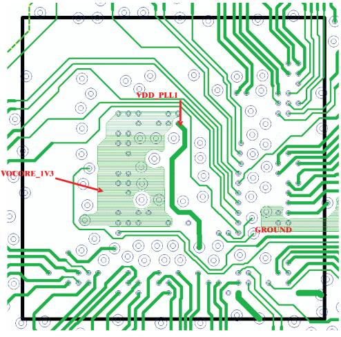
Figure 21. Close-Up of BeagleBoard Layer 3 - Internal Signal
