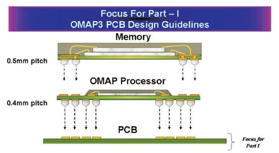
Figure 2 shows a 0.4mm pitch processor and its matching memory at 0.5mm pitch.
