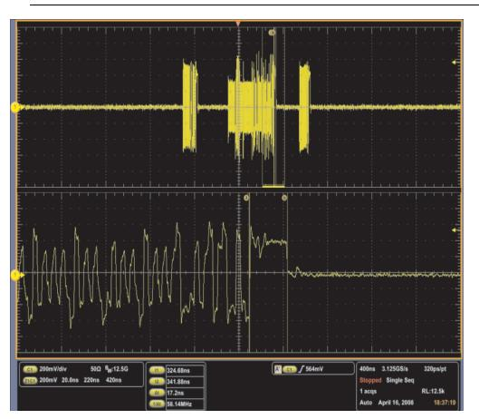
Figure 12. EOP Field of Non-SOP Packet of the Data Packet of the Status Stage of the GET DESCRIPTOR Command
