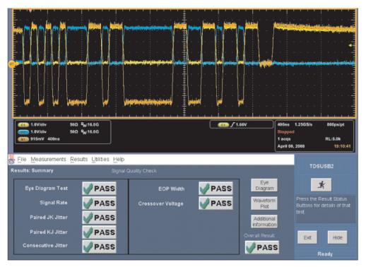
Figure 22. Full-Speed Downstream Signal Quality Test
