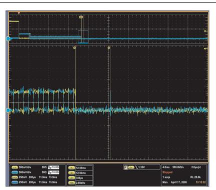
Figure 17. Time Between First SOF and Last Chirp-(J or K)
