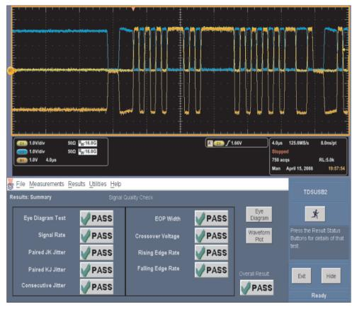
Figure 26. Low-Speed Downstream Signal Quality Test
