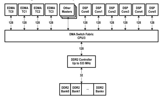
Multiple masters access the DDR2 SDRAM through the DMA switch fabric. If multiple masters access it at the same time, it is arbitrated at the DDR2 controller based on the priority of the masters.
