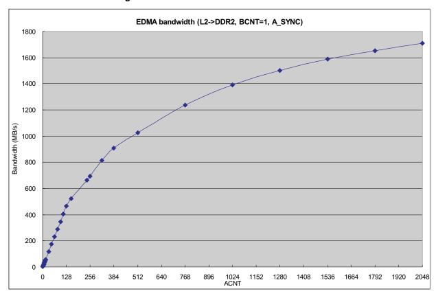
Figure 18. Effect of ACNT on EDMA Bandwidth
