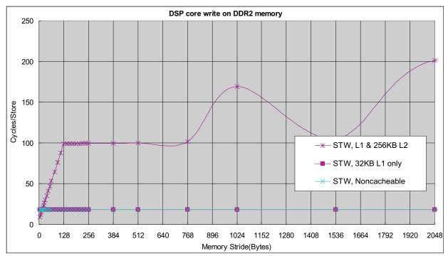
Since the L1D cache is not a write-allocate cache and the cache is flushed before this test, it has no effect on write operation. Therefore, the 32KB L1-only case and non-cacheable case are overlapped in Figure 17.
