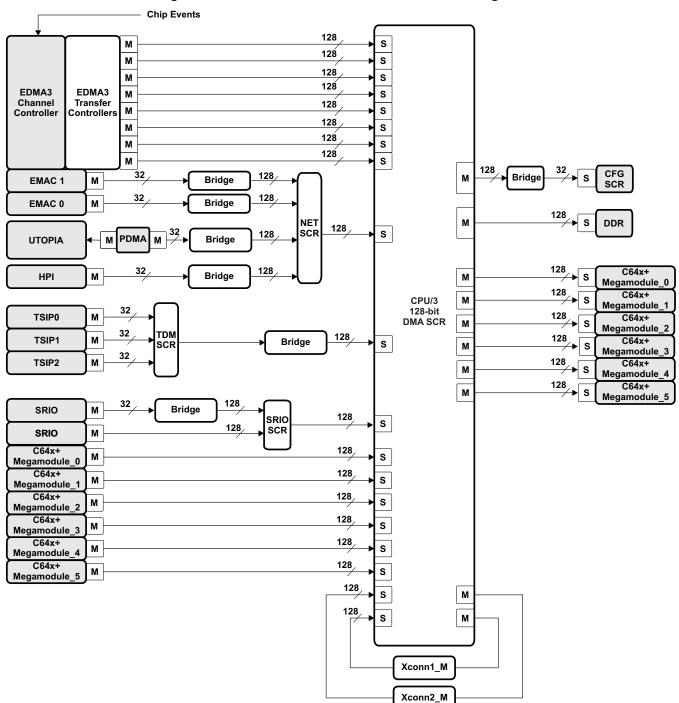
Figure 2. DMA Switched Central Resource Block Diagram
