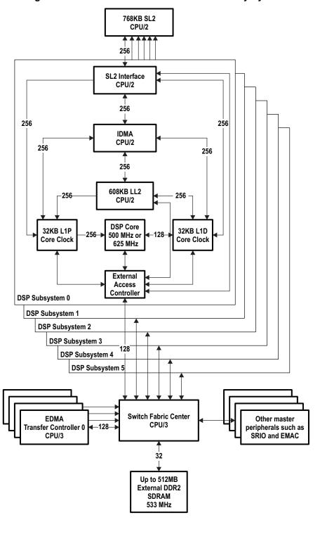
Figure 10. TMS320C6472/TMS320TCl6486 Memory System
