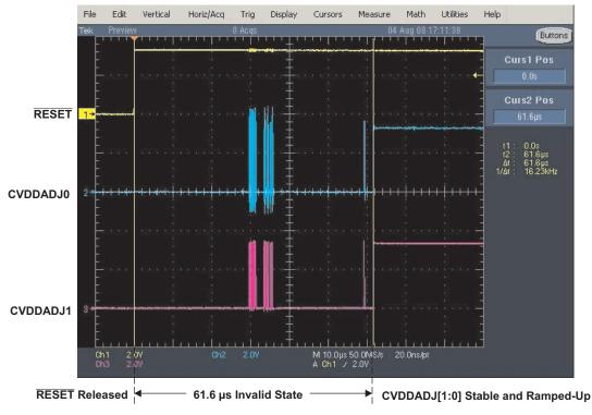
Figure 3. Behavior of CVDDADJ[1:0] Following the Release of RESET
