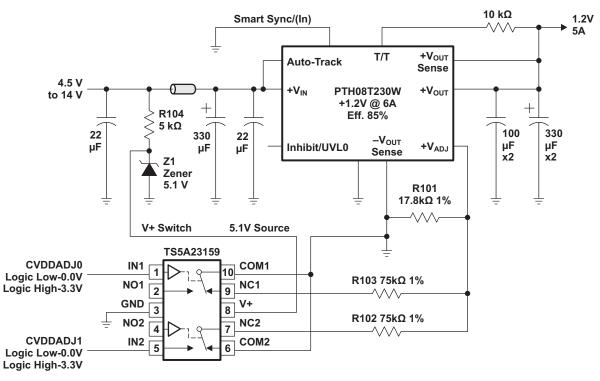
Figure 4. SR Power Supply Reference Design (Core)
