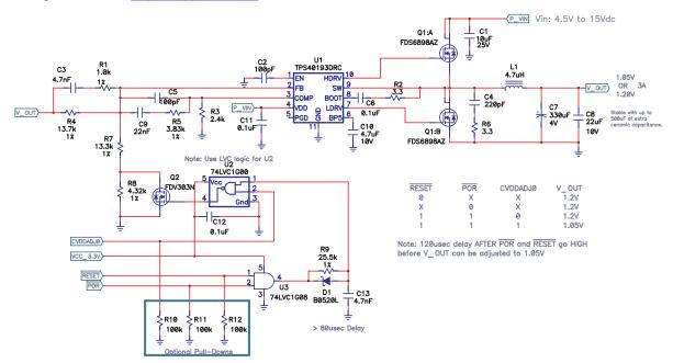
Figure 6. SR Power Supply Reference Design With Pulse Gating (Core)
