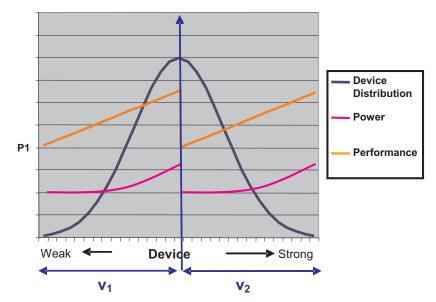
Figure 2. Maximum Performance and Power Consumption with SmartReflex Enabled
