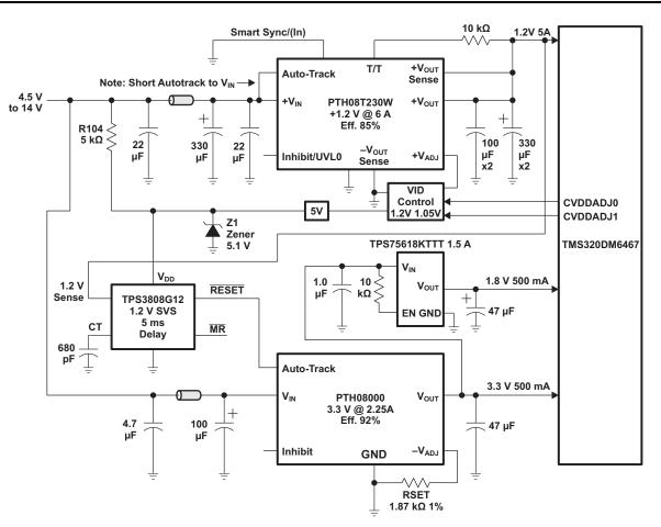
Figure 5. SR Power Supply Reference Design (Complete System)
