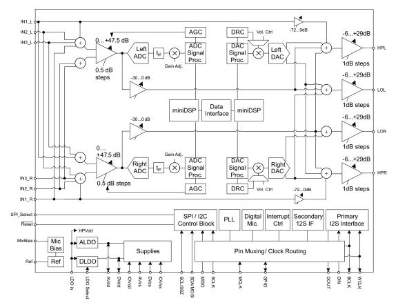
Figure 7. Block Diagram of TLV320AIC3254
