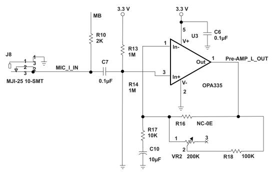
Figure 5. Pre-Amplifier Stage With Gain 31
