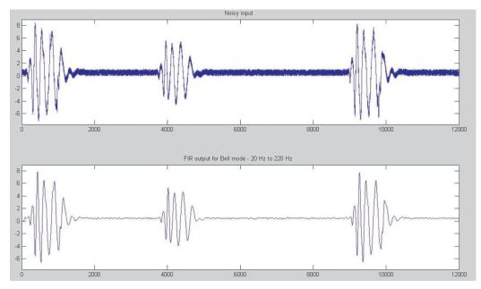
Figure 11. Signal Before and After FIR Filter for Bell Mode
