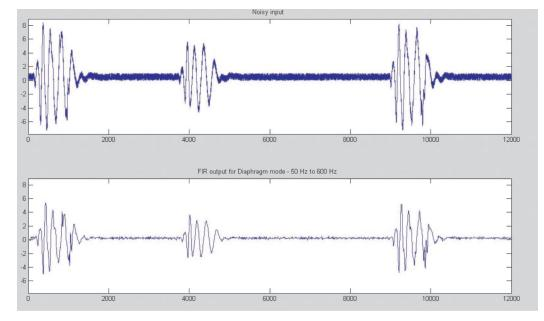
Figure 12 shows the sound waveform before and after applying the filter for the diaphragm mode.
