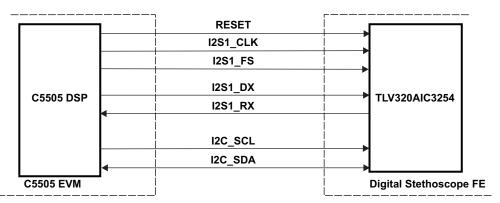
Figure 8 shows the AIC3254 interfaced to the C5515 DSP.
