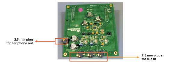
Figure 2. Digital Stethoscope Front-End Board
