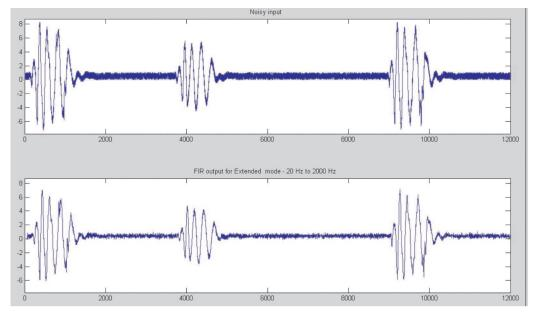
Figure 13. Signal Before and After FIR Filter for Extended Mode
