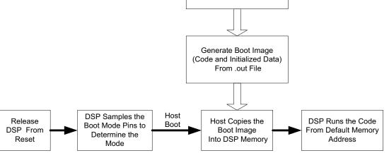
The problem is how to load the code into DSP memory. The .out file (COFF format) generated by Code Composer Studio (CCS) cannot be loaded into DSP memory directly, because it contains application code and initialized data (which is needed to run the DSP standalone) along with information for debugging and linking.
