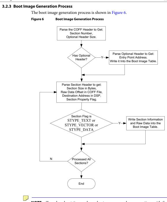
**NOTE**—To reduce boot time and save host memory, only copy sections with the STYPE\_TEXT, STYPE\_VECTOR, or STYPE\_DATA flag into the boot image.
