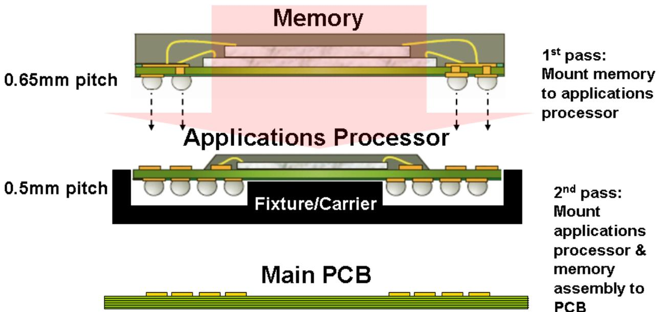
Figure 4. Two-Pass Assembly
