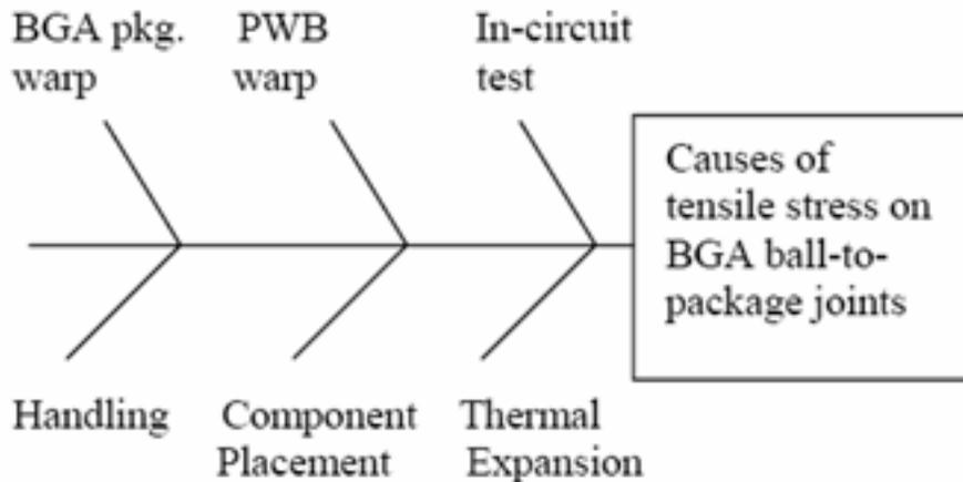
**Figure 11. Causes of Stress on BGA Packages and Solder Joints**
