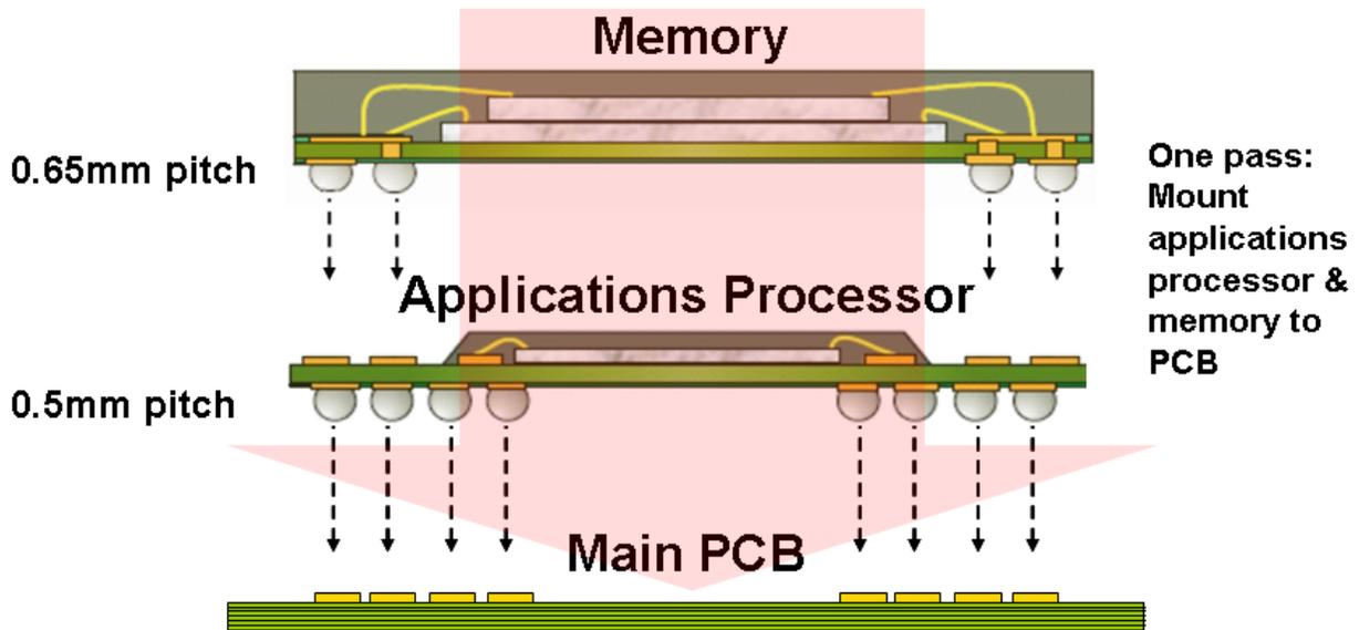
Figure 3. One-Pass Assembly
