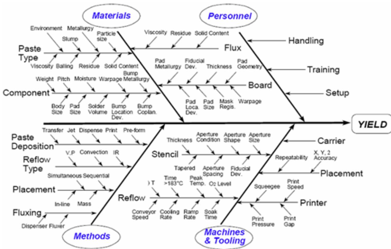
Figure 12. Fishbone Diagram Highlighting Various Causes and Effects Surrounding Assembly Yield
