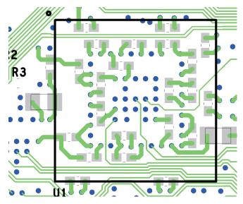
The majority of the components within the U1 outline (which is not physically present on the bottom silkscreen) are bypass capacitors.
