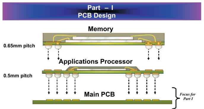
Guidelines for the assembly of PCBs that use PoP technology are covered in the companion article to this document, *PCB Assembly Guidelines for 0.5mm Package-on-Package Applications Processor Part II* (<u>SPRABA8</u>), which is referred to as Part II throughout the remainder of this document. Included are assembly options and suggestions to use when qualifying and working with your assembly vendors.
