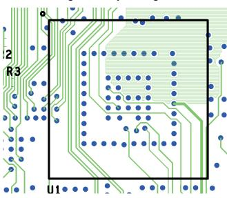
Figure 33. Layer 6 - Signal – Bottom Copper – Bottom Component Outlines
