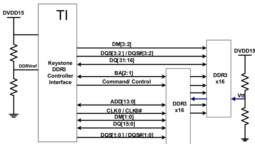
**Figure 6-1. DSP-to-SDRAM Connection Example**
