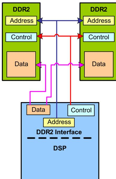
Figure 3-1. Typical DDR Balanced Line Topology
