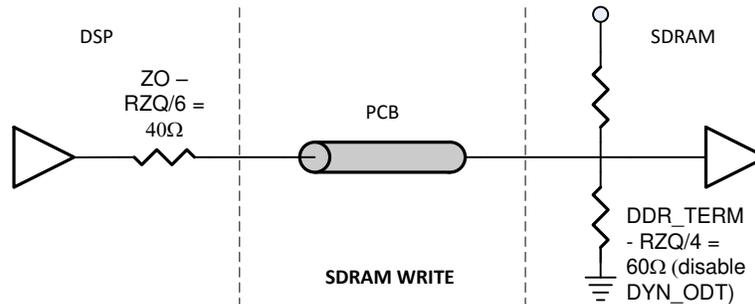
Figure 6-8. Data Group Impedances During Write Cycles on KeyStone II
