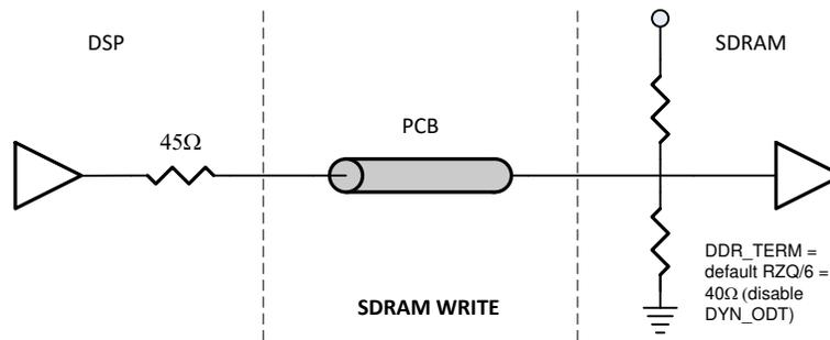
Figure 6-5. Data Group Impedances During Write Cycles on KeyStone I
