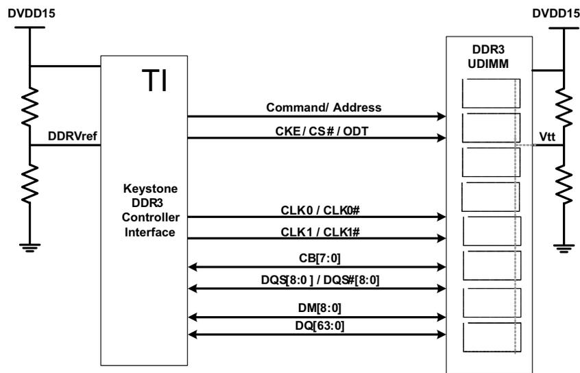
**Figure 6-2. DSP to UDIMM Connection**
