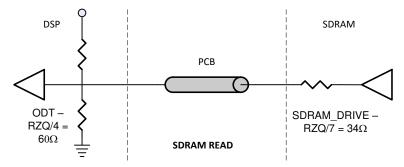
Figure 6-9. Data Group Impedances During Read Cycles on KeyStone II
