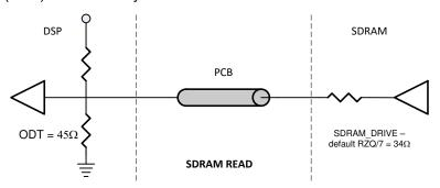
Figure 6-6. Data Group Impedances During Read Cycles on KeyStone I
