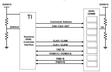
Figure 6-2 shows the basic interconnection between the TI KeyStone DSP and device-specific ECC UDIMM.
