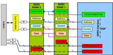
A. The CLKOUT, CS, ODT, and CKE pins will be unique to each rank in a dual rank design.
