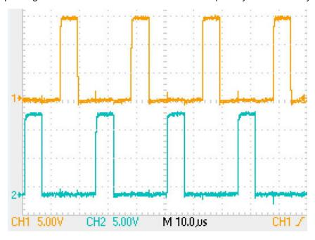
Figure 5-2. Gate Drive Waveforms for the Full Bridge DC-DC Converter
