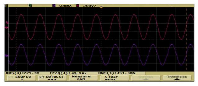
Figure 9-2. Output Voltage and Current (100W Load)
