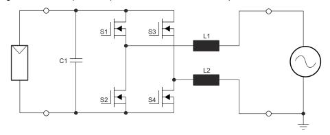
Figure 1-2. Transformerless Inverter Technology
