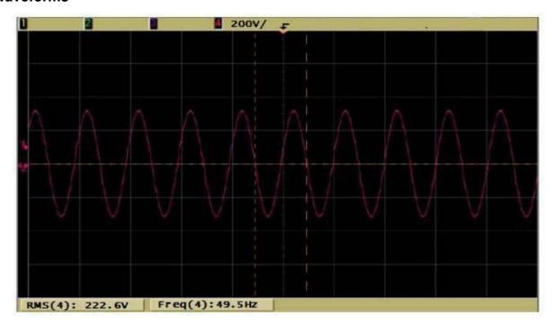
Figure 9-1. Output Voltage at No Load
