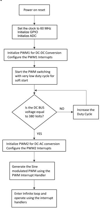
Figure 8-1. Firmware Flowchart
