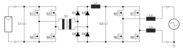
Figure 1-3. High-Frequency Inverter Technology
