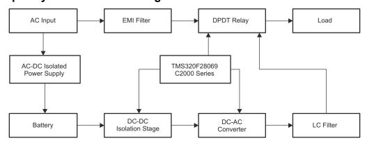
Figure 2-1. High-Frequency Inverter – Block Diagram
