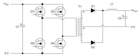
Figure 3-3. Full Bridge Converter
