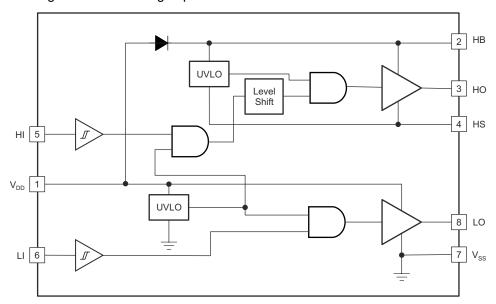
Figure 5-1. Functional Block Diagram of UCC27211
