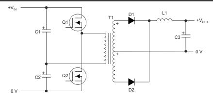
Figure 3-2. Half Bridge Converter
