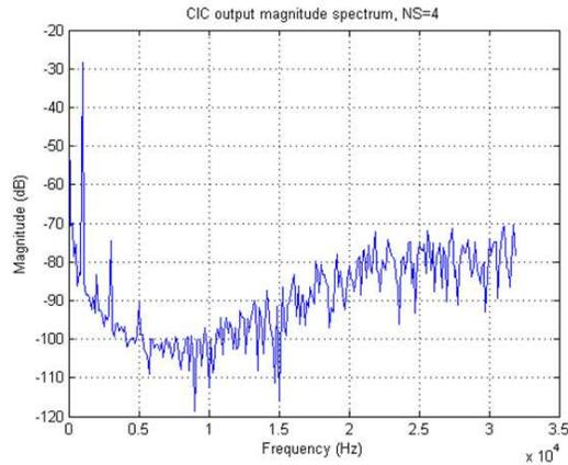
Figure 5. CIC Output With Significant Noise Spectrum Removed
