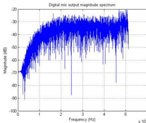
**Figure 4. 1 kHz Tone in Baseband is Difficult to Observe, But Its Present at About -30 dB Magnitude**
