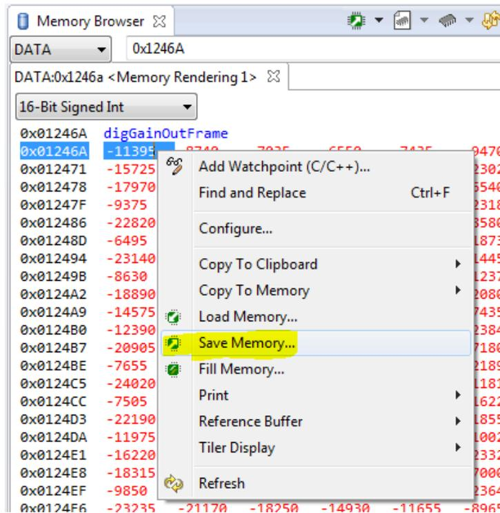
Figure 20. Saving the Captured Audio Samples to a .dat File
