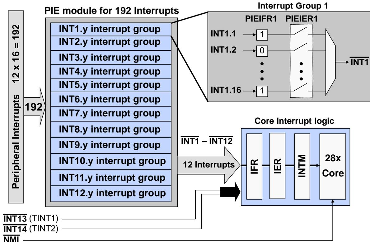
Figure 5. Peripheral Interrupt Expansion (PIE) Module
