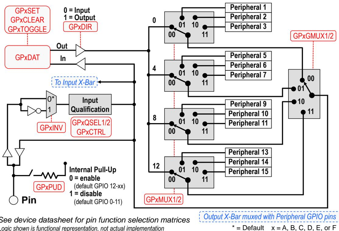
Figure 6. General-Purpose Input/Output (GPIO) Pin Block Diagram
