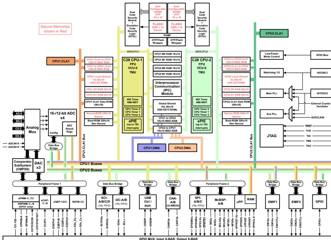
Figure 1. F2837xD Functional Block Diagram
