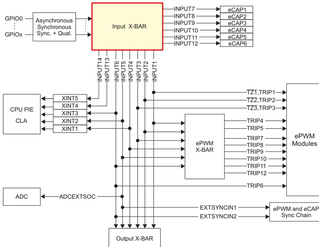
**Figure 7. Input X-BAR**
