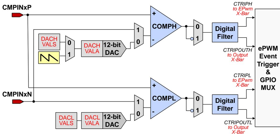
Figure 10. Comparator Subsystem (CMPSS) Block Diagram
