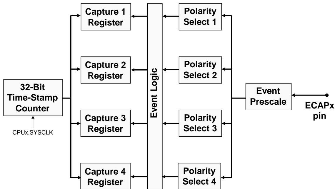
Figure 12. Enhanced Capture (eCAP) Module Block Diagram
