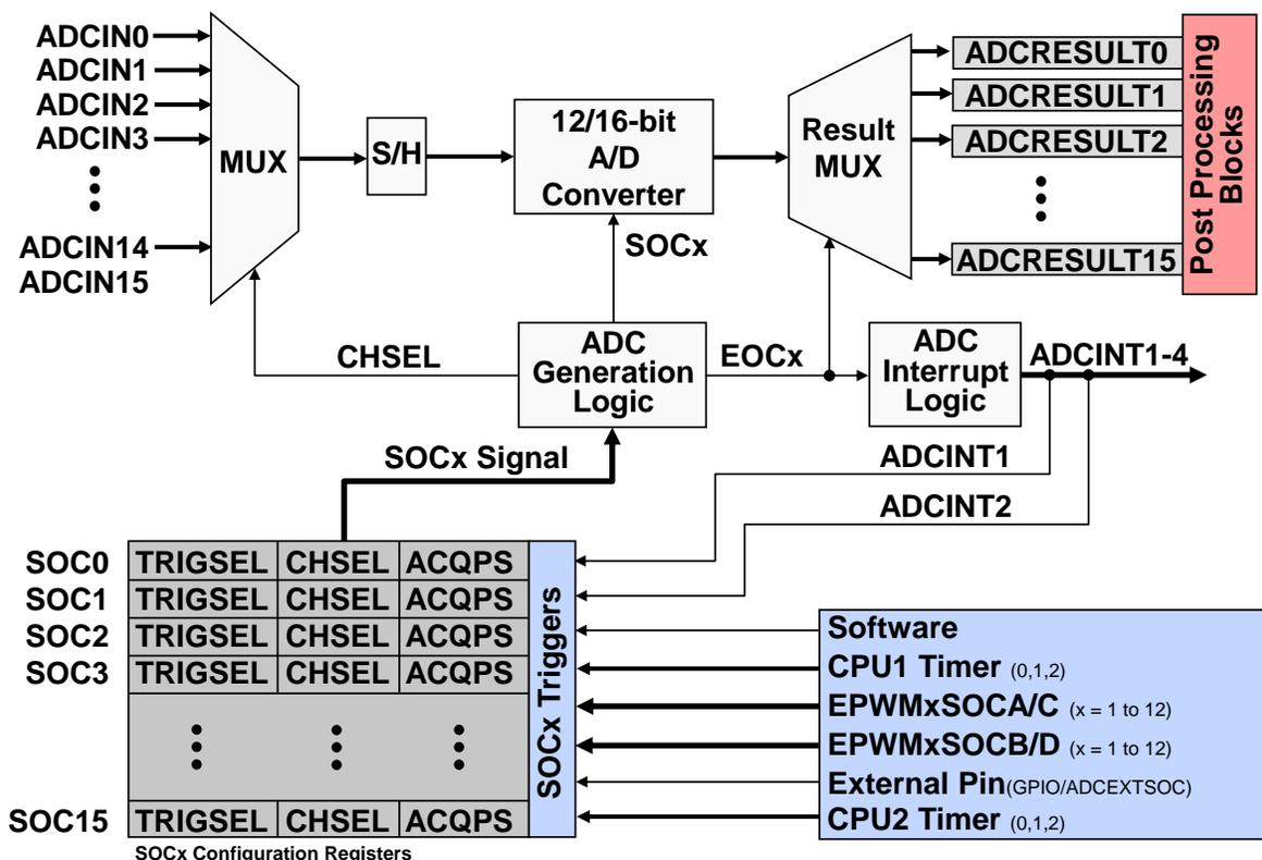
Figure 9. Analog-to-Digital Converter (ADC) Block Diagram
