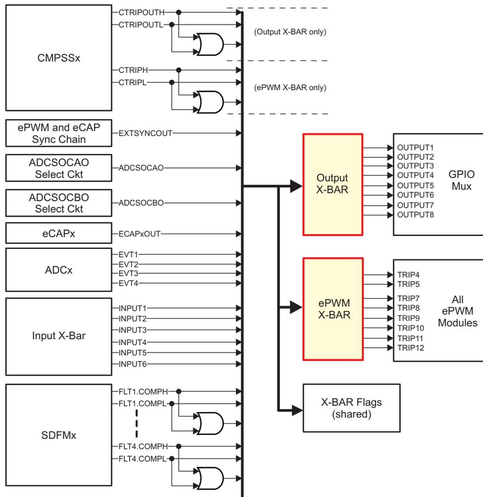
**Figure 8. Output and ePWM X-BARs**
