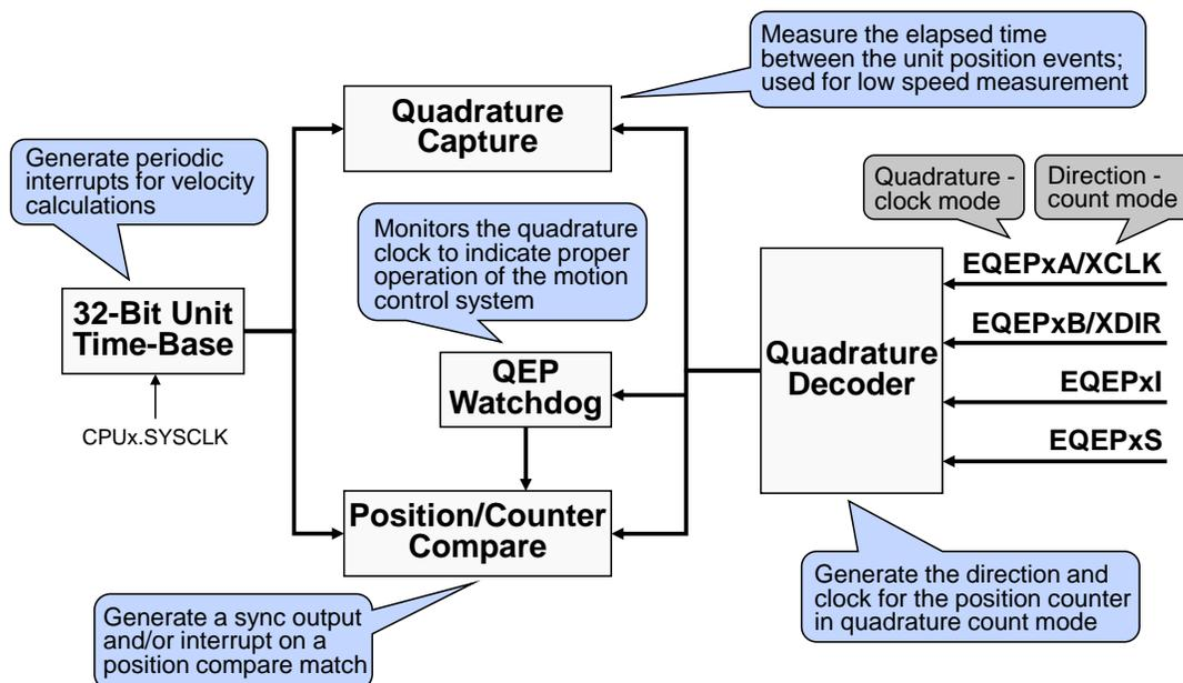
Figure 13. Enhanced Quadrature Encoder Pulse (eQEP) Module Block Diagram
