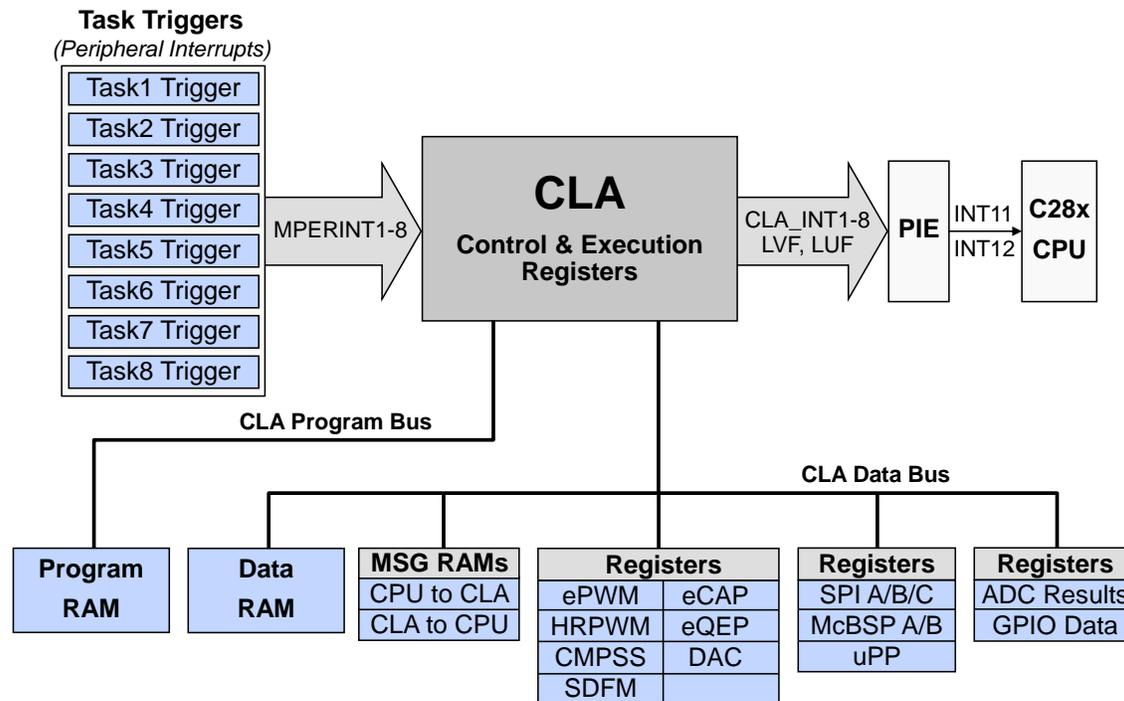
**Figure 14. Control Law Accelerator (CLA) Block Diagram**
