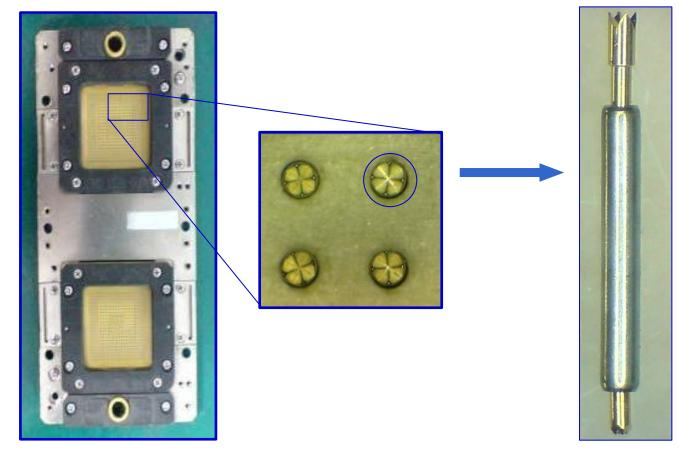
Contactor for 0.8/1.0mm pitch PBGA (23X23)
