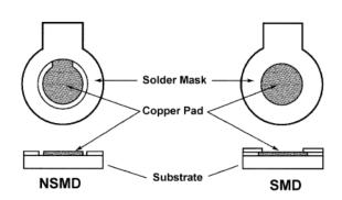
For NSMD pads, TI recommends a clearance (typically 3 mils) between the copper pad and solder mask to avoid overlap between the solder joint and solder mask due to mask registration tolerances.
