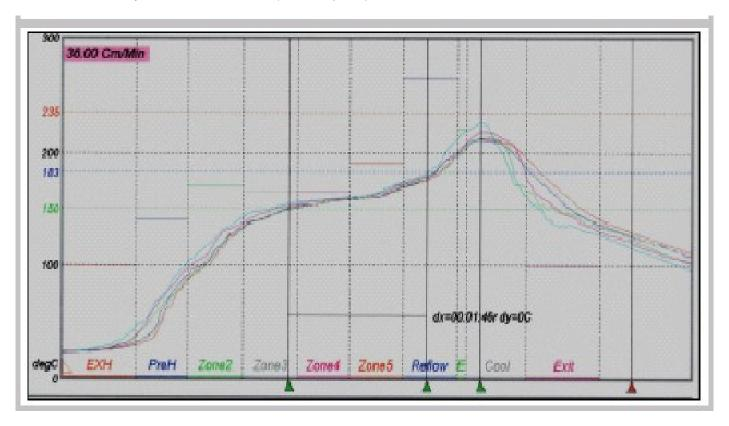
PbSn Reflow Profile: Time between 150°C – 170°C: 100 sec Time above 183C: 60 sec Peak Temp: 220C
