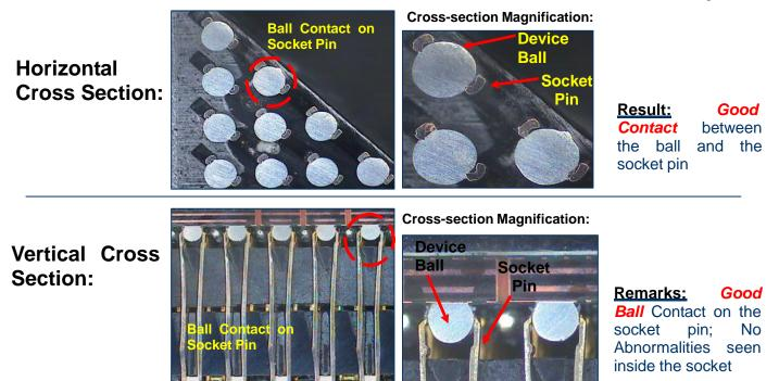
The witness marks left on the solder ball from the contact are shown below. There is no damage to the bottom of the ball and typical pin contact signature is seen in the ball marking magnification photograph below.
