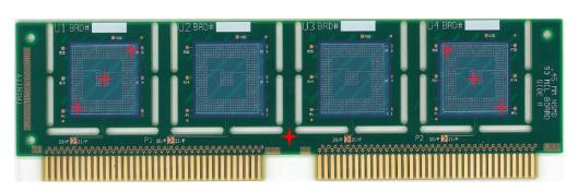
Thermocouples were attached to the solder joint through the other side of the board by drilling through the PCB. Then the components were placed on the board.
