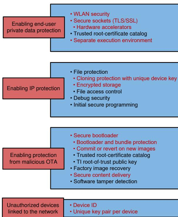
**Figure 6-5. E-Lock Security Challenges and SimpleLink™ Wi-Fi Security Enablers**
