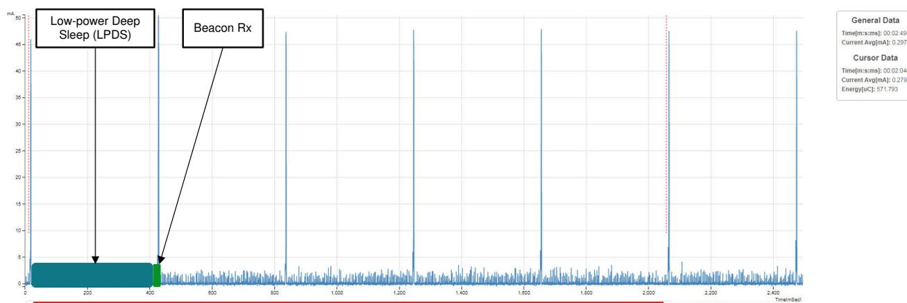
**Figure 6-4. Always Connected Idle Current With LSI = 500 milliseconds**
