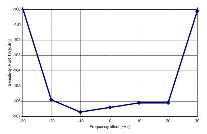
Figure 4. 4.8 kbps, MDMCFG2.DEM\_DCFILT\_OFF = 0
