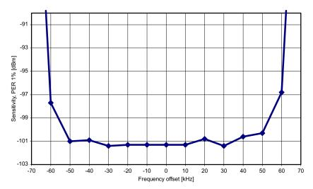
Figure 8. 38.4 kbps, MDMCFG2.DEM\_DCFILT\_OFF = 0
