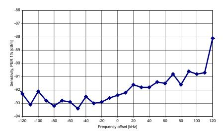
Figure 11. 250 kbps, MDMCFG2.DEM\_DCFILT\_OFF = 1
