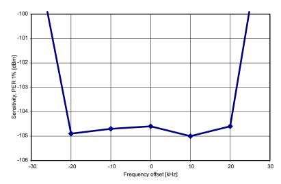
Figure 5. 4.8 kbps, MDMCFG2.DEM\_DCFILT\_OFF = 1
