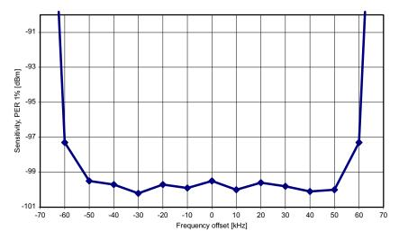
Figure 9. 38.4 kbps, MDMCFG2.DEM\_DCFILT\_OFF = 1
