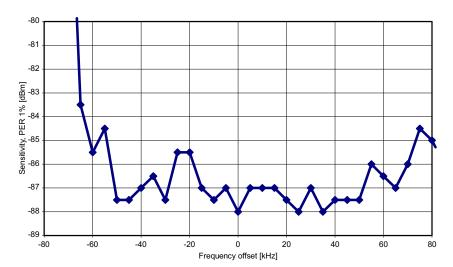
Figure 12. 500 kbps, MDMCFG2.DEM\_DCFILT\_OFF = 0
