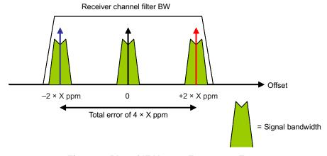
Figure 1. Plot of IF Versus Frequency Error
