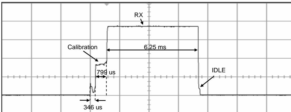
**Figure 10. Current Consumption (EVENT1 = 3 and RX Timeout = 6.25 ms)**
