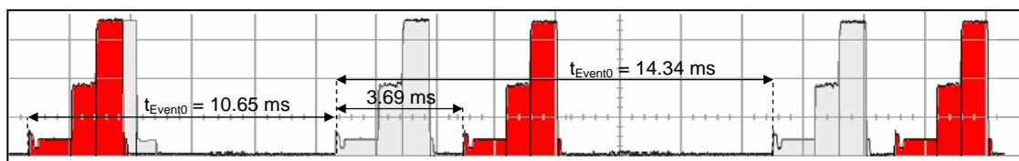
**Figure 6. Current Consumption vs. Time ( $t_{Event0} = 10.65 \text{ ms}$ )**
