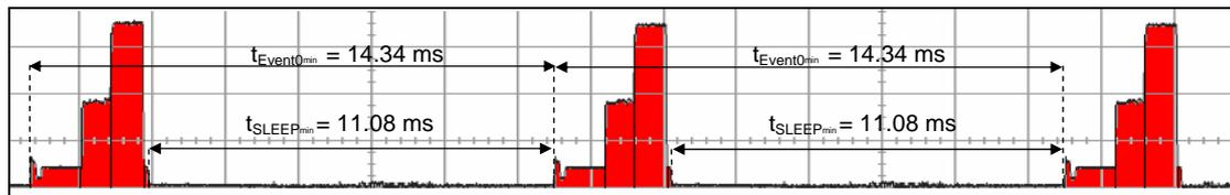
**Figure 4. Current Consumption vs. Time (No Packets Received)**
