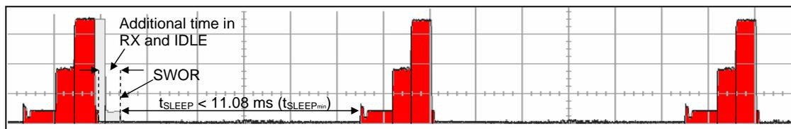
**Figure 5. Current Consumption vs. Time (One Packet Received)**
