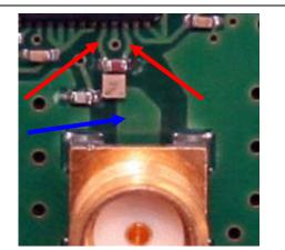
Figure 6 Differential (red) connecting lines and single ended (blue) connecting line
