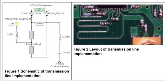
The transmission line implementation shown in Figure 1 and Figure 2 is straight forward and employs only four discrete components. However the PCB real estate taken up is significant and the performance is sensitive to changes of line width of the 180° transmission line, PCB thickness and variation in the PCB material.
