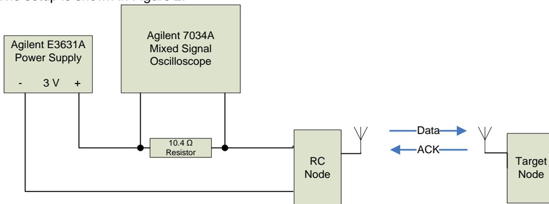
Figure 2. RC Active Current Measurement Setup
