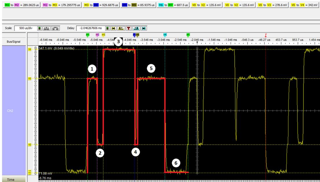
Figure 5. RC TX w/o ACK Current Waveform
