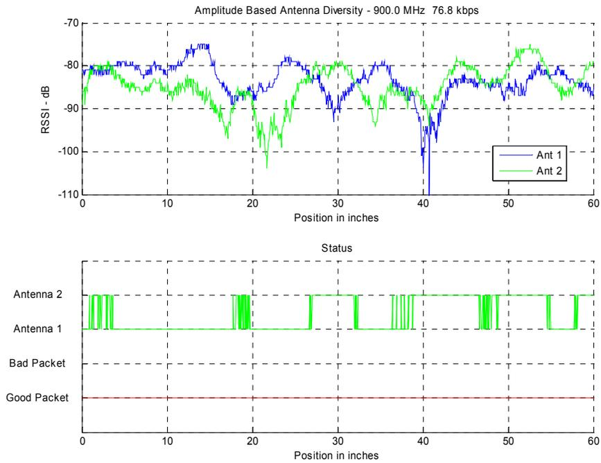
Figure 7 - Amplitude Based Antenna Diversity, 900 MHz, 76.8 kbps
