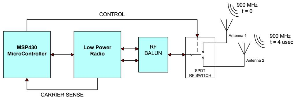
Figure 2 - Single Radio Amplitude-Based Antenna Diversity
