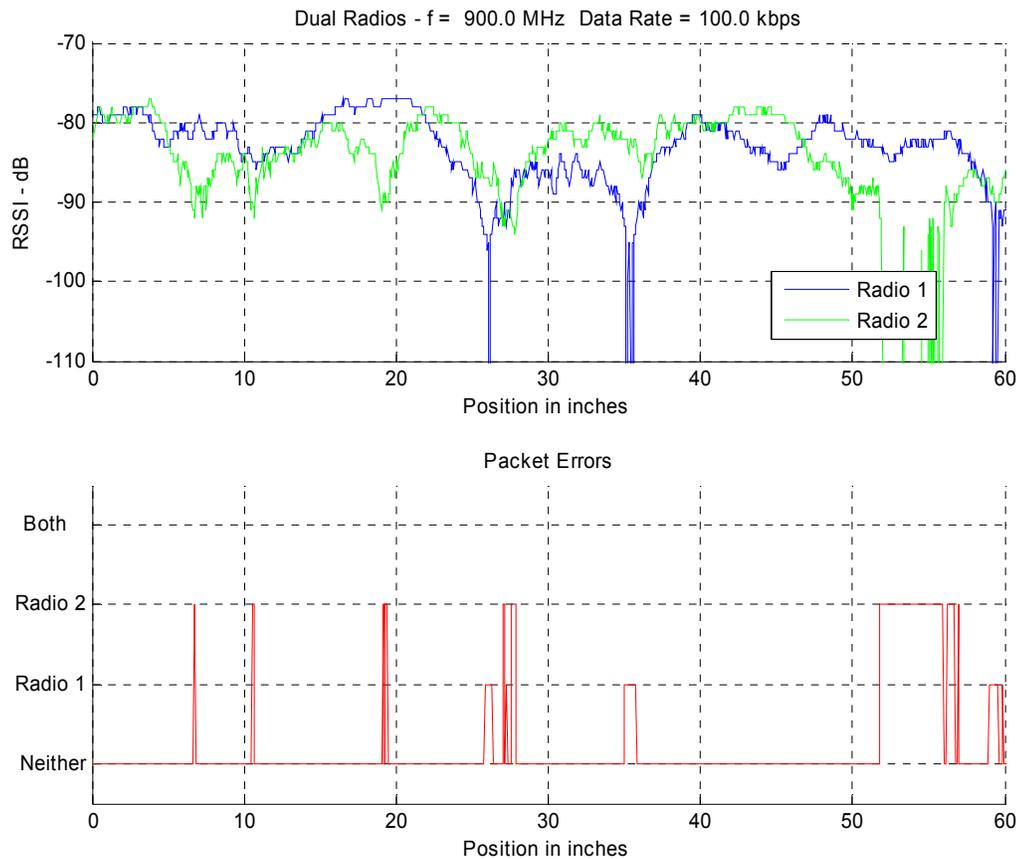
**Figure 12 - Dual Radios, 900 MHz, 100 kbps**
