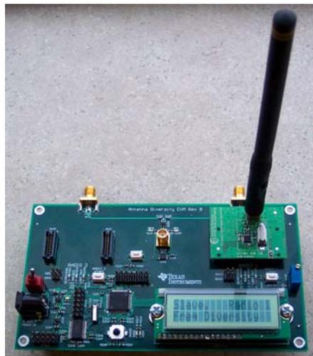
**Figure 8 - Antenna Diversity EVM, Rev B. One Radio. One Antenna, Frequency Diversity Mode**
