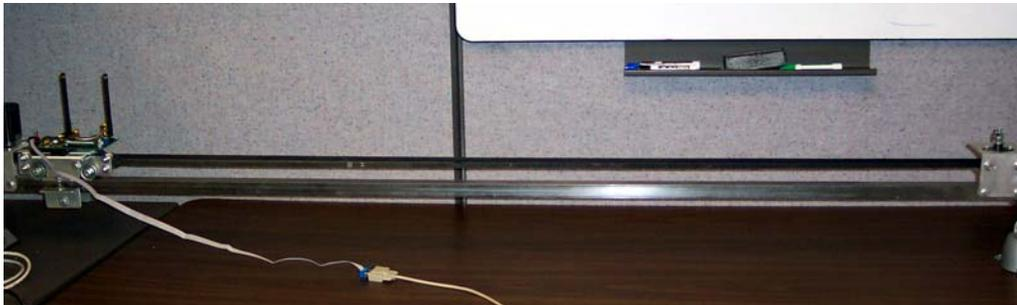
Figure 5 - 60 inch Linear Actuator with EVM
