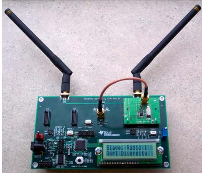
Figure 6 - Antenna Diversity EVM, Rev B. One Radio Amplitude Based Antenna Diversity Mode
