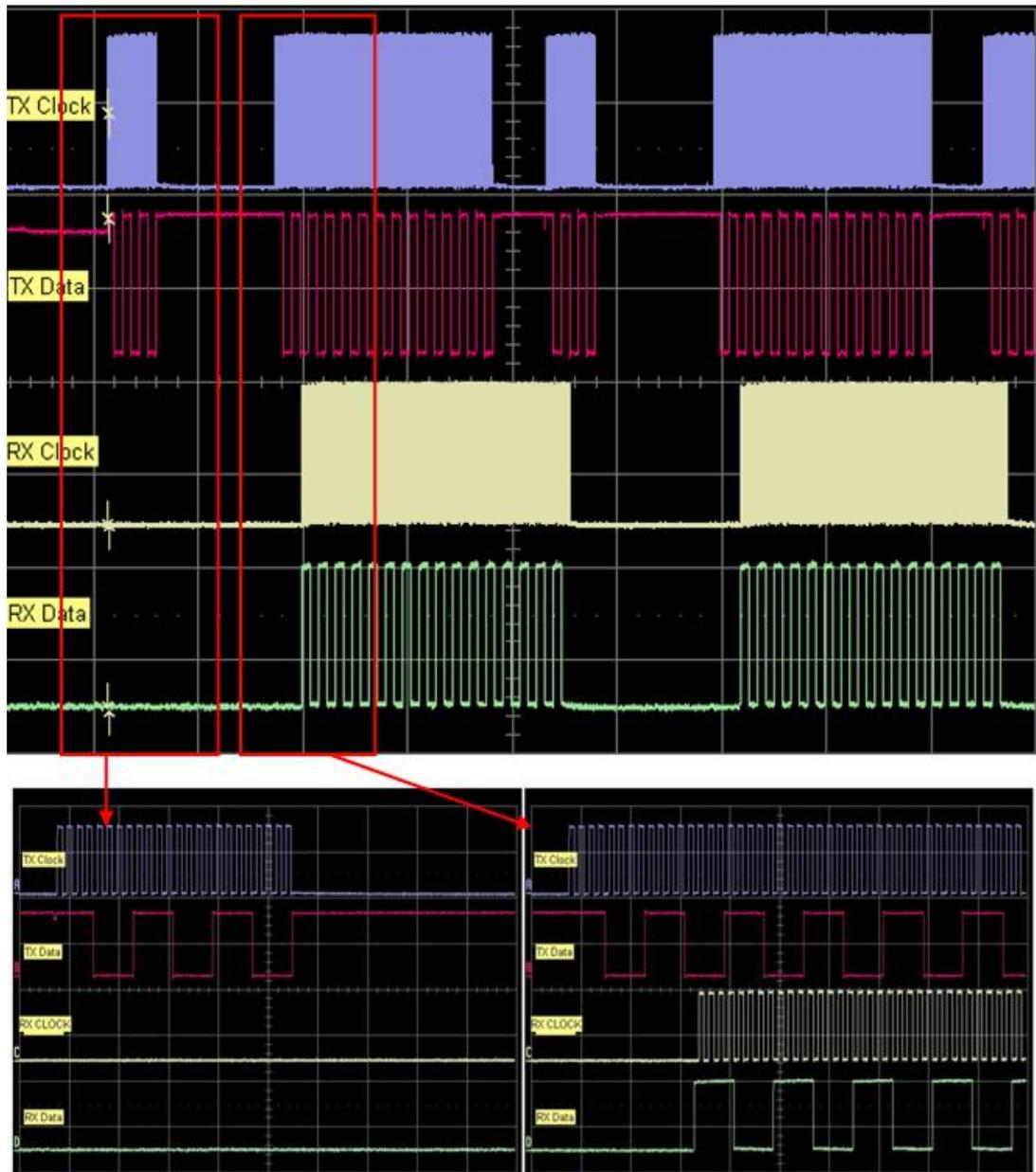
**Figure 3. Voltage Transitions on the Clock and Data Pin for the Transmitter and Receiver configured in Serial Synchronous Mode with packet handling hardware enabled.**
