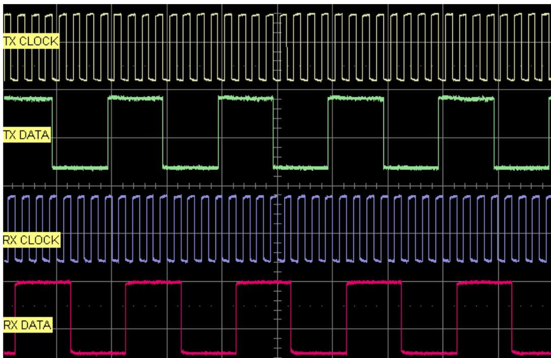
Figure 5. Voltage Transitions on the Clock and Data Pin for the Transmitter and Receiver Configured in Serial Synchronous Mode with Packet Handling Disabled.
