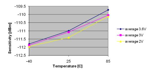
Figure 4.2. Typical Sensitivity vs. Temperature and Power Supply Voltage, 38.4 kbps
