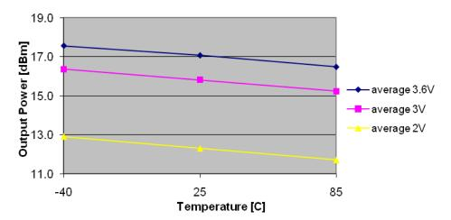
Figure 4.7. Typical Output Power vs. Temperature and Power Supply Voltage. PA\_CFG2 = 0x7F
