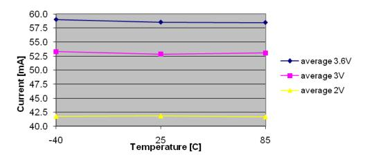
Figure 4.8. Typical TX Current vs. Temperature and Power Supply Voltage. PA\_CFG2 = 0x7F
