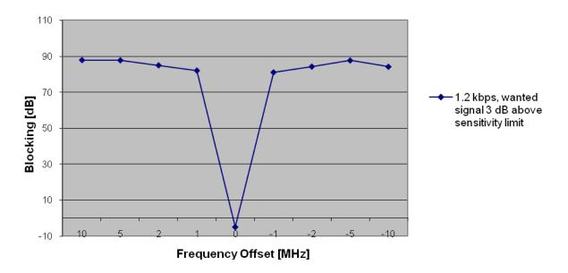
Figure 4.5. Typical Blocking 1.2 kbps, Unmodulated Interferer
