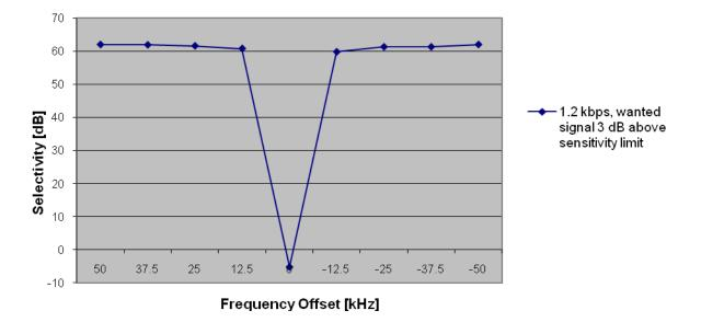
Figure 4.4. Typical Selectivity, 1.2 kbps, Unmodulated Interferer
