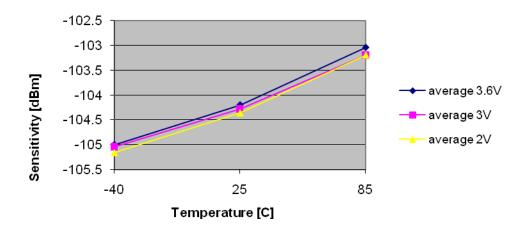
Figure 4.3. Typical Sensitivity vs. Temperature and Power Supply Voltage, 200 kbps
