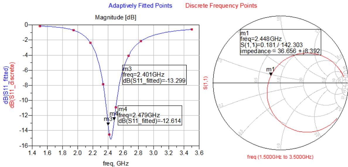
Figure 7. S11 Looking into the Curved Dipole with Added Ground Plane
