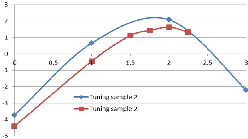
Figure 9. TRP (in dBm) versus the Number of Notches Cut (x-axis)
