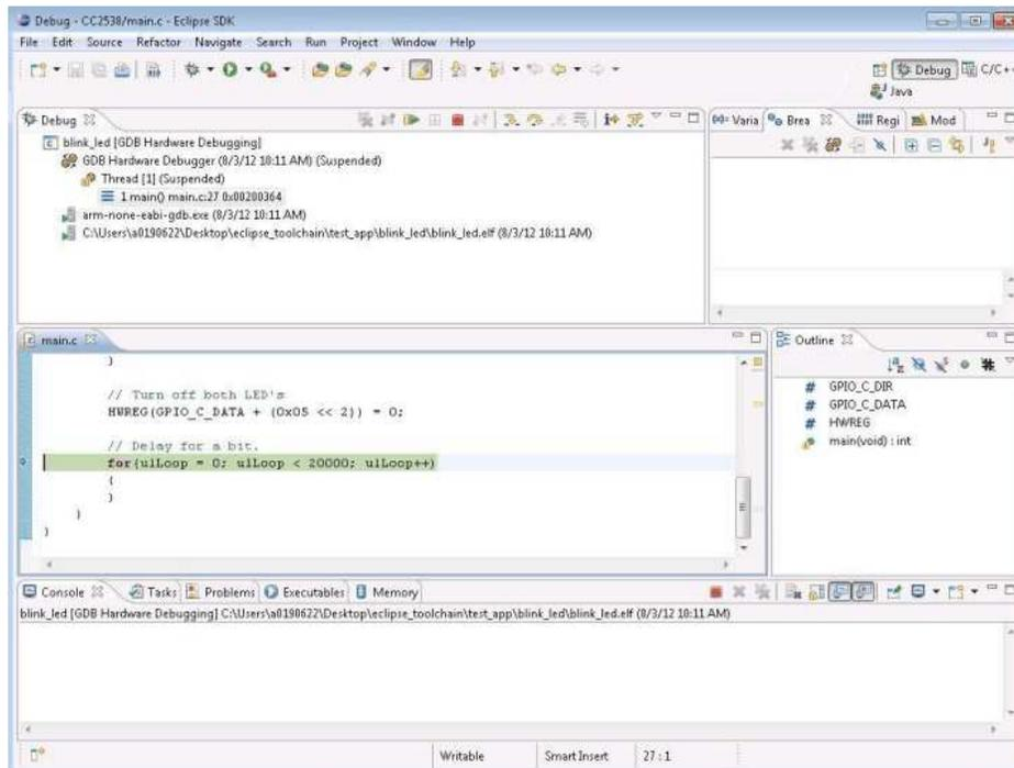
**Figure 23. Running the Software Example From Debugger**
