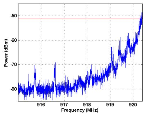
Figure 5. Spurious Emission 915 MHz - 920.4 MHz
