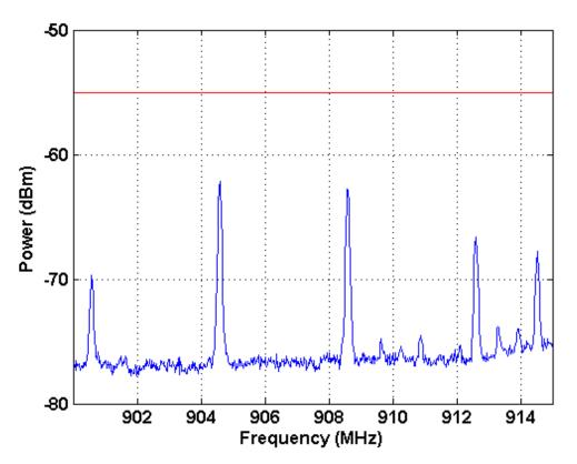
Figure 4. Spurious Emission 900 MHz - 915 MHz
