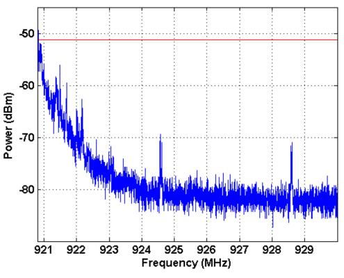
Figure 6. Spurious Emission 920.8 MHz - 930 MHz
