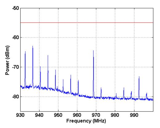
Figure 8. Spurious Emission 930 MHz - 1000 MHz
