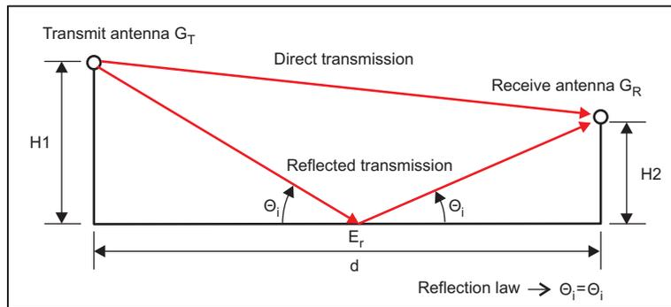
Figure 1. Transmission With Ground
