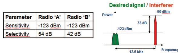
Figure 5. Weak RF Interferer Level of – 90 dBm
