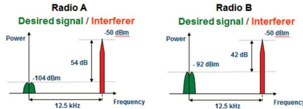
Figure 6. Strong RF Interferer Level of - 50 dBm
