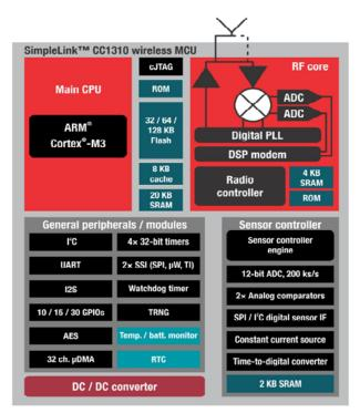
Figure 2. CC1310 Block Diagram
