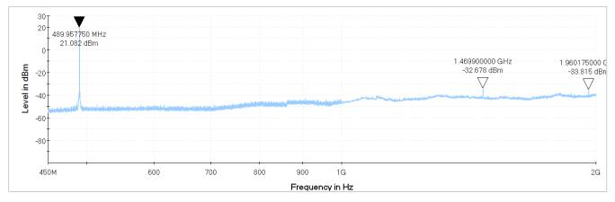
Figure 5. Tx Spectrum Plot at 21 dBm Peak EIRP and Whip Antenna
