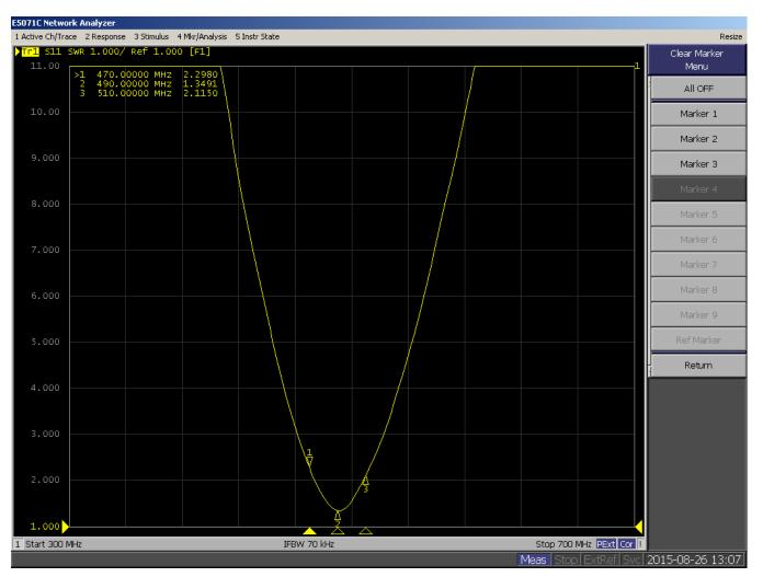
Figure 9. Antenna Bandwidth at VSWR: 2
