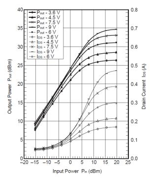
Figure 7. Increasing Power Supply to the MOSFET
