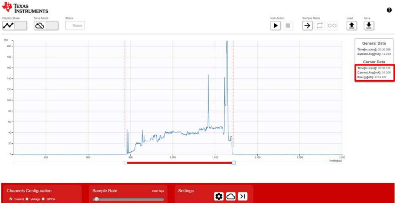
Figure 16. Average Current Measurement With IMETER-BOOST Device
