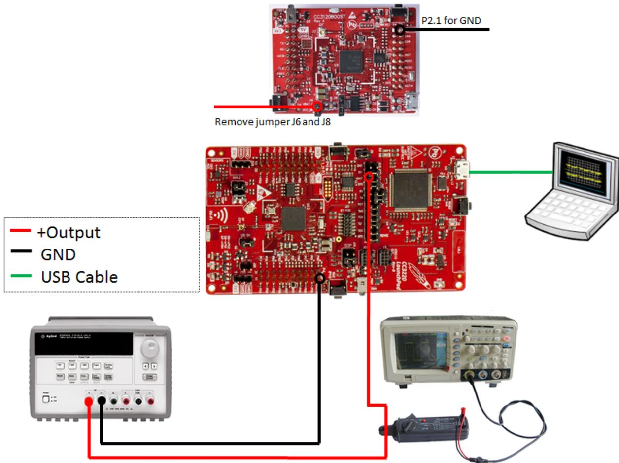
**Figure 17. Oscilloscope With Current Probe Test Setup**
