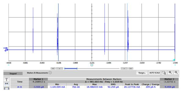
Figure 9. ZED Current Consumption Measurement in Sleep Mode
