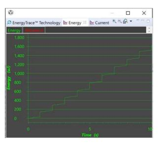
Figure 16. ZED EnergyTrace Energy Measurement
