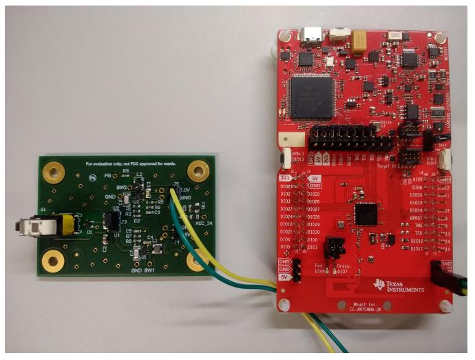
Figure 18. LAUNCHXL-CC26x2R1 LaunchPad Connected to TIDA-00690 Reference Design PCB
