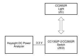
Figure 2. Measurement Setup Overview
