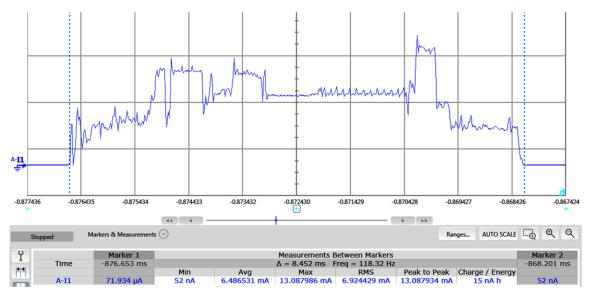
Figure 11. ZED Current Consumption Measurement for One On/Off Toggle Operation (5 dBm)
