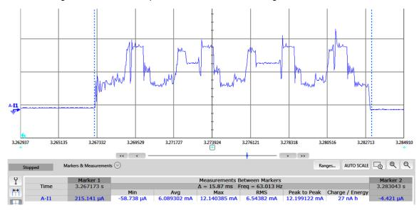
Figure 13. GPD Current Consumption Measurement for Sending GPDF With 3 Duplicates (5 dBm)
