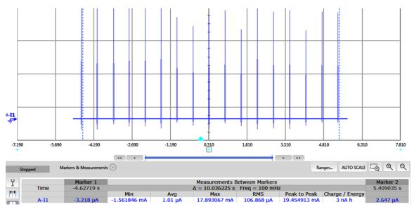
Figure 12. GPD Current Consumption Measurement in Sleep Mode
