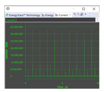
Figure 15. ZED EnergyTrace Current Measurement
