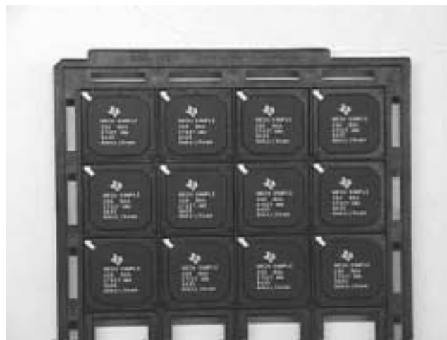
Figure 2. Matrix Tray With Devices in Place
