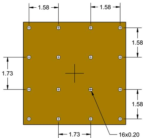
Example Via Layout Design Via layout may vary depending on layout constraints (Note D, F above)
