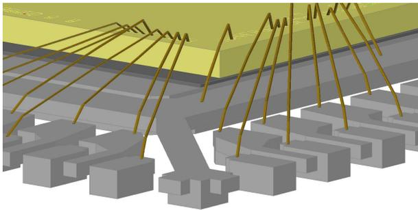
The MRQFN Package maximum thickness is 0.80 mm. The package seating height will be dependent upon the solder paste volume and land pad design.
